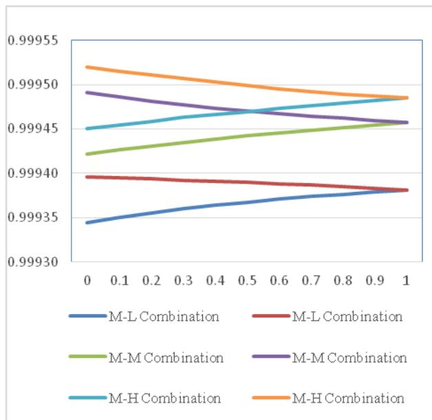
Fig. 6: System availability variation for Medium values of unsuccessful rates and repair rates (Low (L), Medium(M) and High(H))
