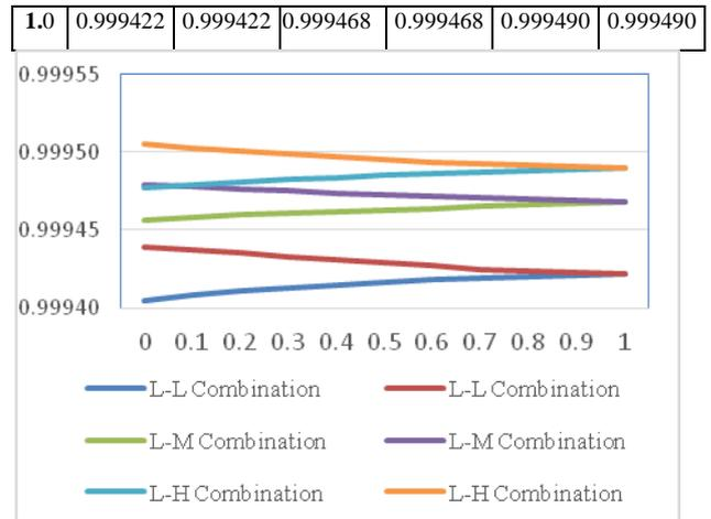
Fig. 5: System availability variation for Medium values of unsuccessful rates and repair rates (Low (L), Medium(M) and High(H))
