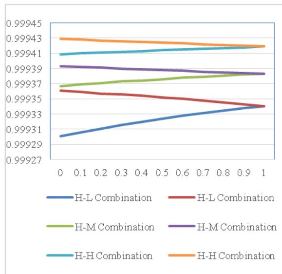
Fig. 7: System availability variation for High values of unsuccessful rates and repair rates (Low (L), Medium(M) and High(H))
