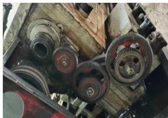
Fig. 2. Actual Image of Feed drive mechanism in Lathe machine
