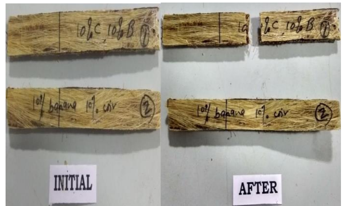
FIGURE 5. FLEXURAL TESTING SPECIMEN
