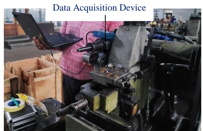
Figure 3: Acquiring vibration signatures with accelerometer
