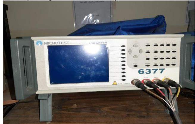
Figure 2. MICROTTEST impedance analyzer 6377
