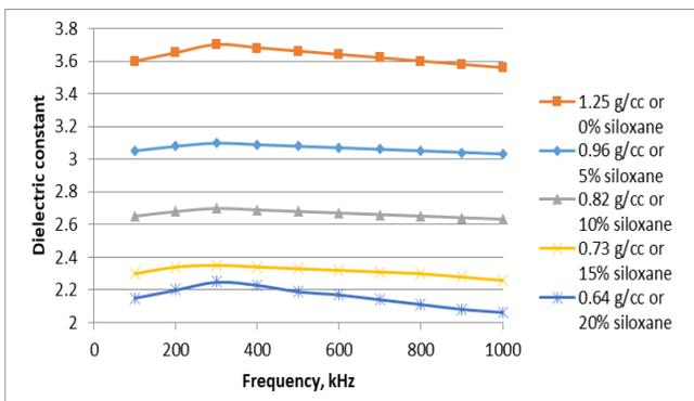
Figure 5. Variation of dielectric constant values for selected specimens
