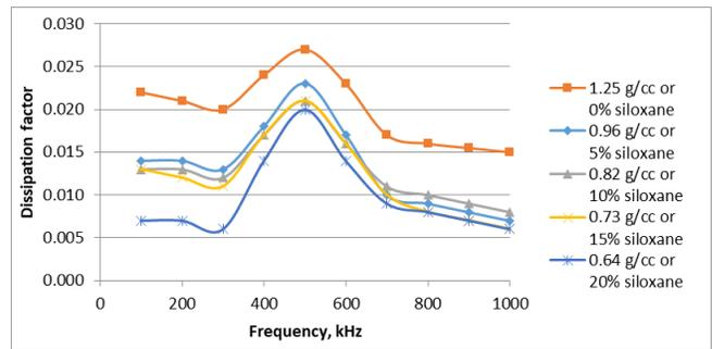
Figure 7. Variation of dissipation factor values for selected specimens
