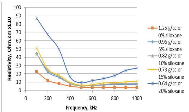
Figure 6. Variation of resistivity values for selected specimens
