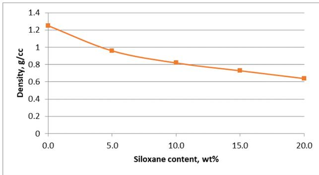
**Figure 3.** Density of the epoxy as a function of siloxane content
