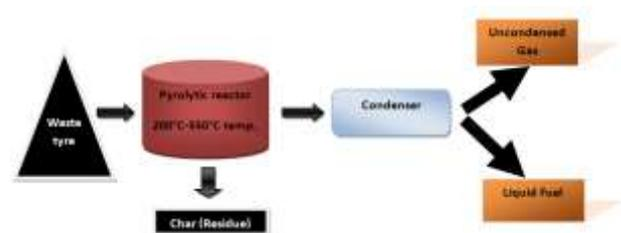
Fig. 1 Schematic diagram of pyrolysis process.
