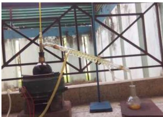
Fig. 3 Test set-up for Distillation of crude WTPO.
