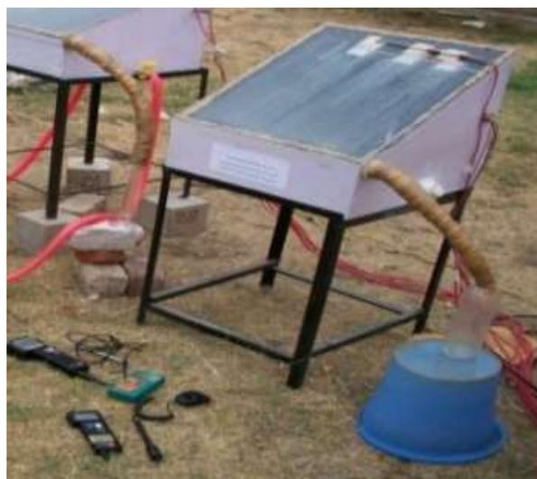
Fig.2. Photograph of the SSSS configuration
