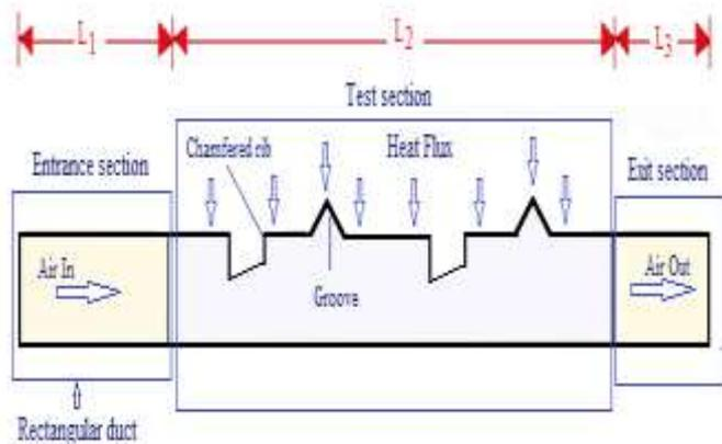
Fig.1: 2D Computational Domain for solar air heater
