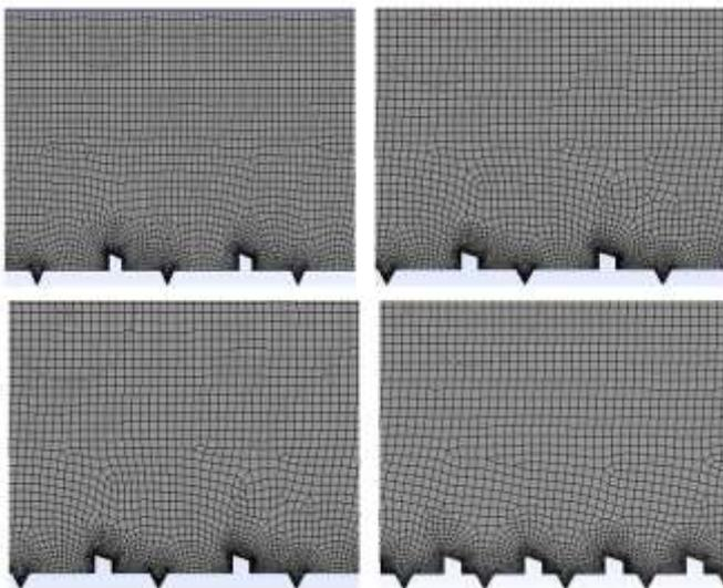
Fig.3: 2-dimensional meshing of transverse chamfered rib groove, for different value of pitch, and relative, groove, position
