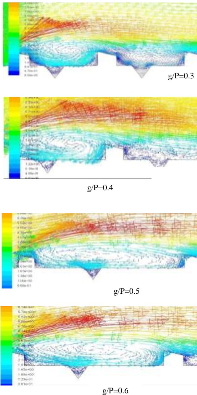
Fig. 5: Images of the Velocity' vector and velocity' magnitude at different groove; positions ( $g/P$ )
