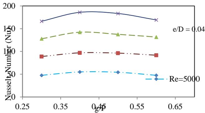
Fig: 8: Effect of  $g/P$  on  $Nu$  for entire range of  $Re$  at  $P/e = 6$ ,  $e/D_h = 0.04$  and  $\phi = 18^\circ$
