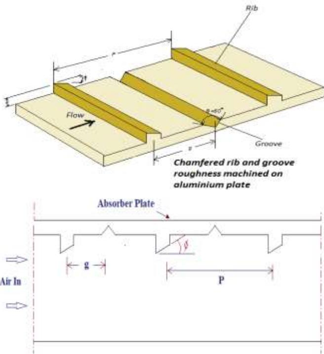
Fig.2: Schematic Sketch diagram of Chamfered Rib Geometry
