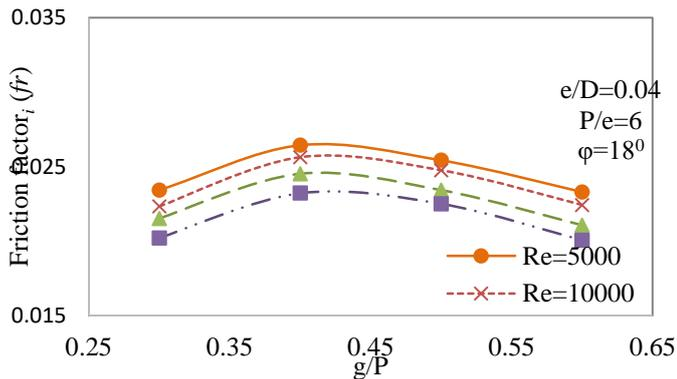
Fig: 9: Effect of  $g/P$  on  $f_r$  for entire range of  $Re$  at  $P/e = 6$ ,  $e/D_h = 0.04$  and  $\phi = 18^\circ$
