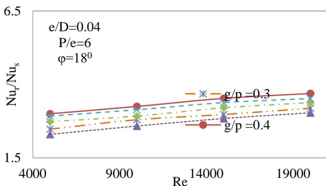
Fig: 10: Effect of  $g/P$  on Nusselt<sub>*i*</sub> number enhancement ratio ( $Nu_i/Nu_s$ ) at  $\phi = 18^\circ$
