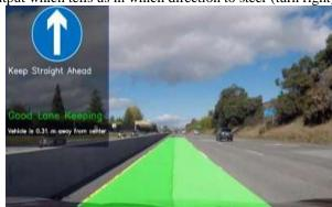
Output which tells us to go straight is the road is straight. It also tells us how far we are from the center of the lane and warns us if we deviate.
