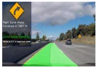
Output which tells us in which direction to steer (turn right)
