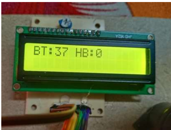
Fig 13 Body temperature displaying on lcd
