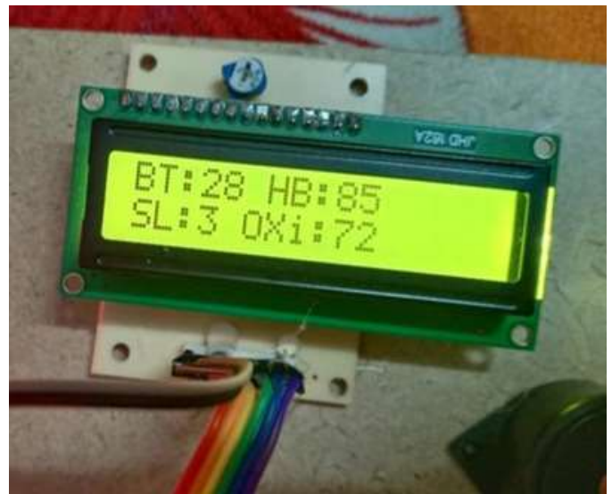
Fig 6 heart beat sensor values displays on lcd
