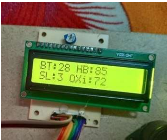
Fig 9 Displaying oxygen levels on lcd
