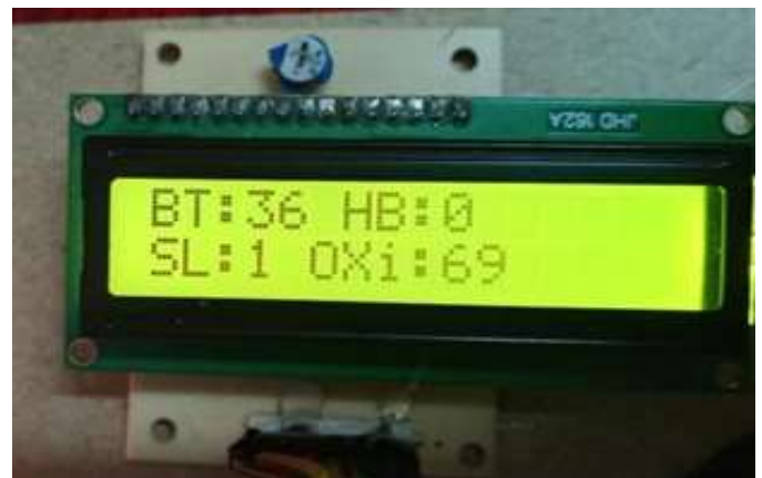
Fig 10 Displaying saline levels in lcd app
