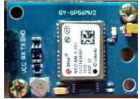
Figure 9 Neo6M GPS module
