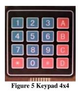
It has a 16 built in Push button contacts in Row and Column lines. It has 8 output terminals where 4 terminals are allocated
