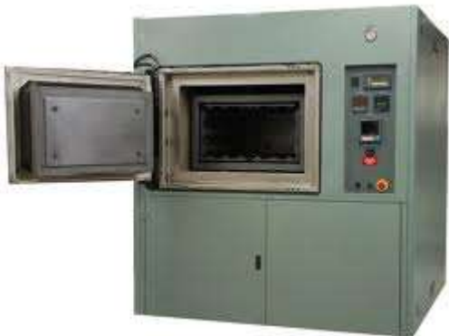
Fig. 11 Vacuum Sintering Furnace
