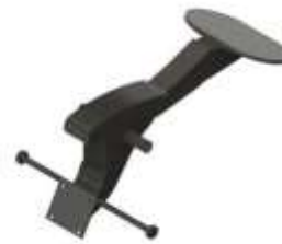
Fig.3. Rear accessory assembly of a two-wheeler modelled in Fusion 360
