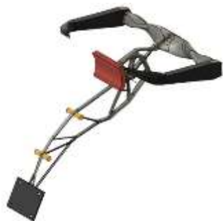
Fig. 5. Converged rear accessory assembly with rear handle, rear indicator and rear side reflector mounts
