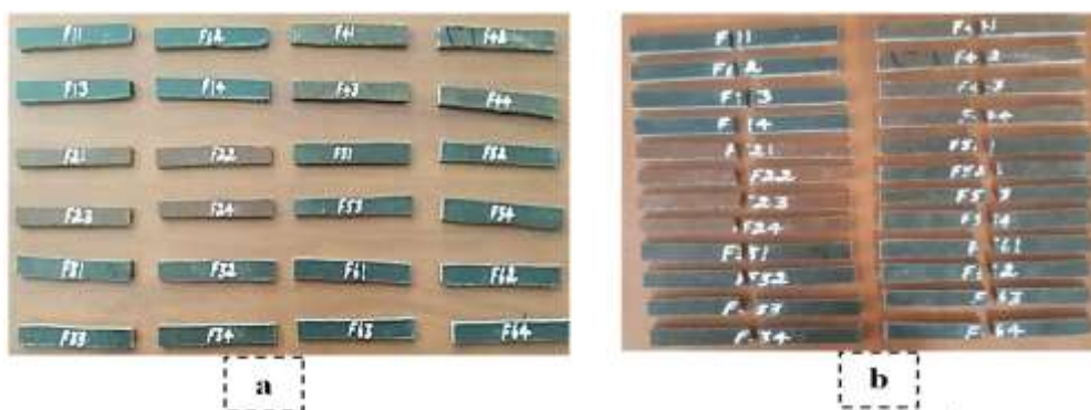
Figure 1 Flexural Test Specimens (A) Before Test (B) After Test
