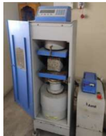
Figure 6 Split tensile strength testing
