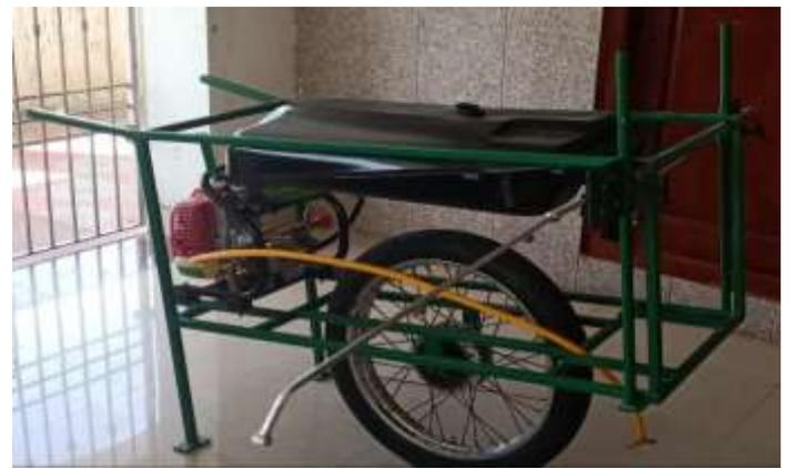
Fig 8 Trolley Encompassed Pesticide Sprayer
