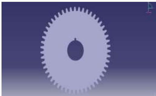
Figure 2 Front View of Spur Gear
