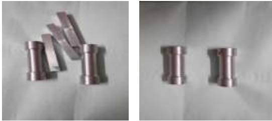
Figure 5 Fabricated Specimen of Al+SiC+B 4 C Composite
