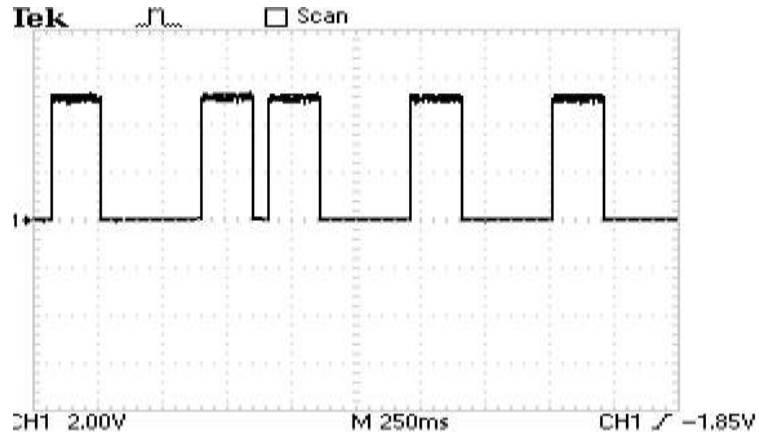
Fig.12.DSO output of Gate pulses for 3volt Bridge
