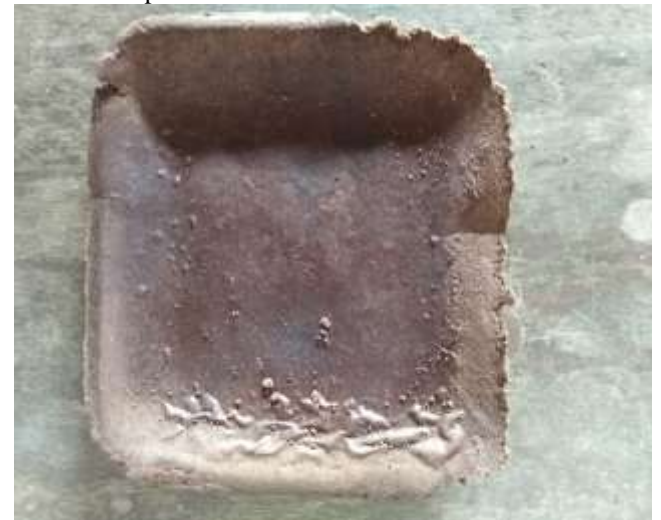
Fig. 3 sample (B) 30% of CSP filled composite
