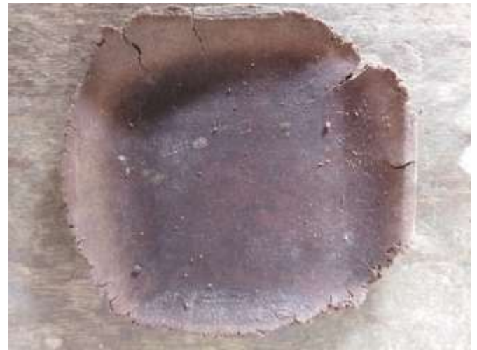
Fig. 2 sample (A) 20% CSP filled composite
