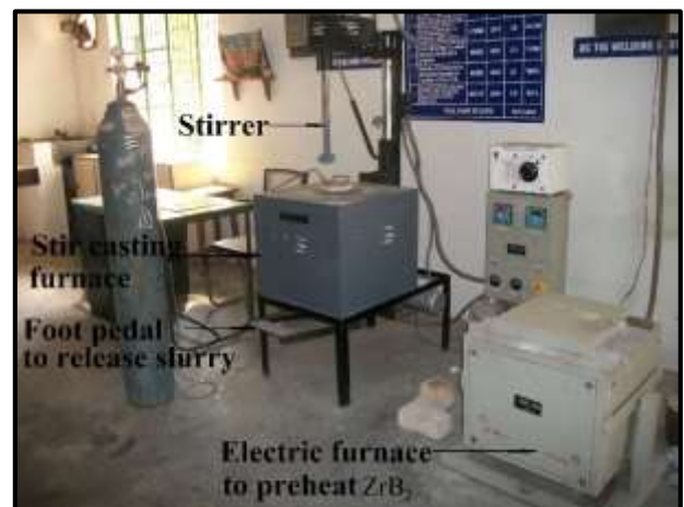
Fig. 1 Electric stir casting furnace employed to fabricate AA7075/ ZrB_2 composites
