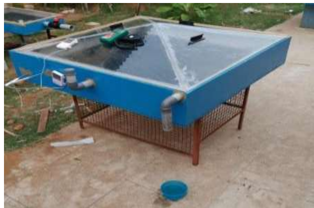
Fig 1: Square pyramid solar still
