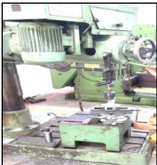
Fig. 2(a) Universal Radial Drilling Machine. Figure 2(b) Experimental setup (high speed 3 axis vertical CNC machine)
