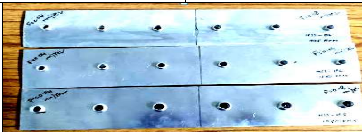
Fig.2(g). Al 6061-T6 Friction drilled with HSS (Ø6mm)
