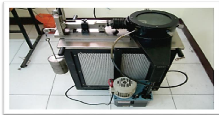
Figure 7. Pin on disk experimental setup
