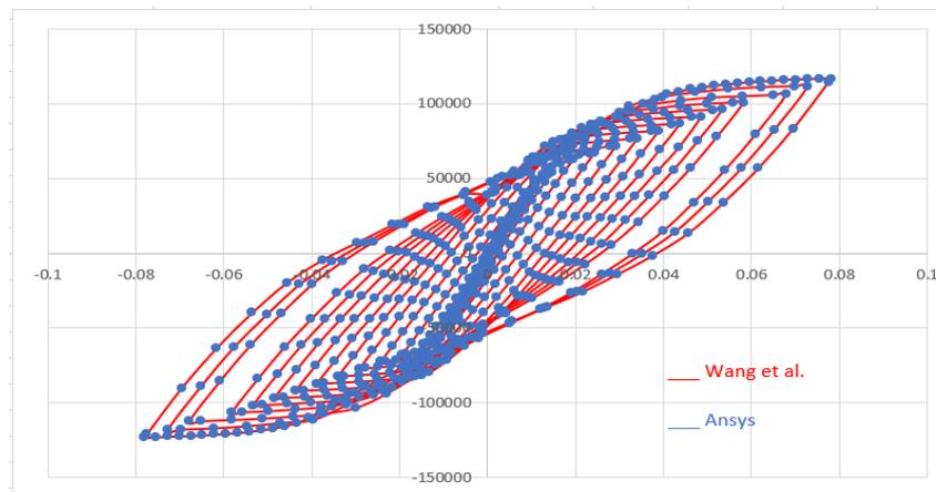
**Fig .3** Hysteresis curve of normal beam
