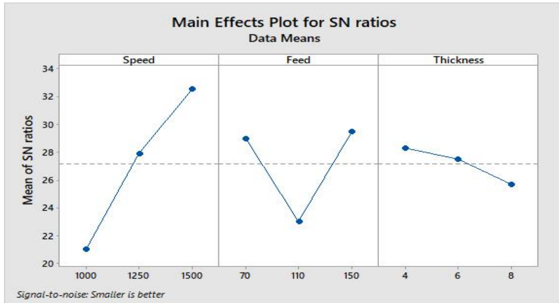
Figure 10 Main effect plot for SN ratios of Circularity
