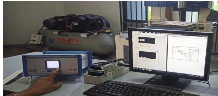
Figure 6 Software and Data Acquisition system for recording the Force & Torque
