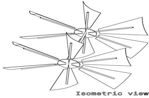
**Figure 1 Isometric view of dual-rotor 6 blade assembly**
