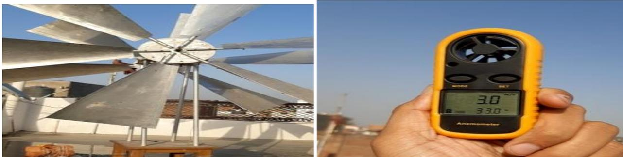
**Figure.4(a) Side view of the real dual rotor assembly, (b) Anemometer wind speed and temperature measuring instrument.**
