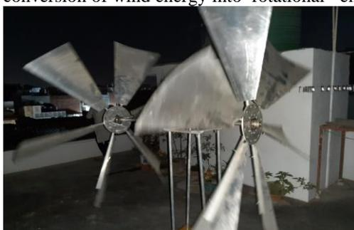
**Figure 5. Real Dual rotor Wind Turbine.**
