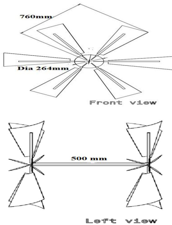
**Figure 3(a), (b). Front view of the blade assembly.Side view coaxial shaft dual rotor.**
