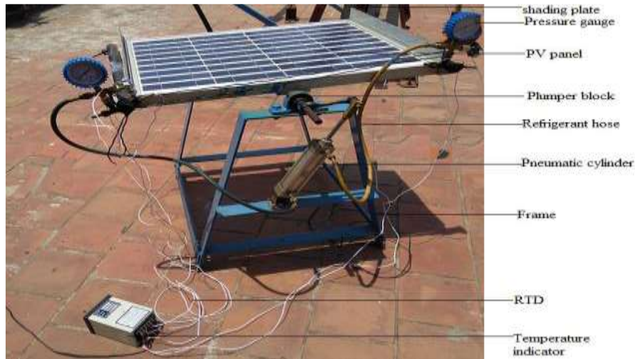
Fig. 1 Proposed Pneumatic Actuator system for Solar PV panel tracking
