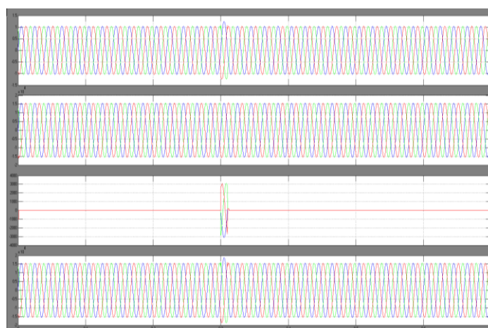
Figure 6: Voltages swell (LLLG Fault) (a) voltage of grid (b) voltage of load (c) compensated voltage (d) PCC voltage
