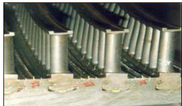
Fig. 2: Assembled guide Blades in Inner Casing
