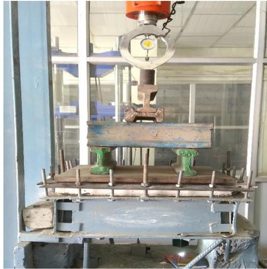
Figure: 1 Loading frame, platform, and proving ring
