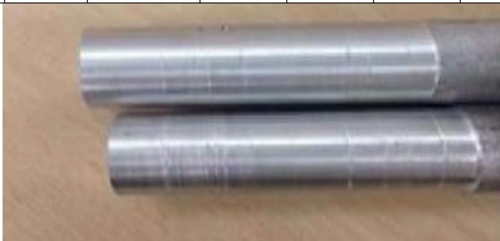
**Figure 1:** AA2219 Aluminum Alloy Matrix Composite
