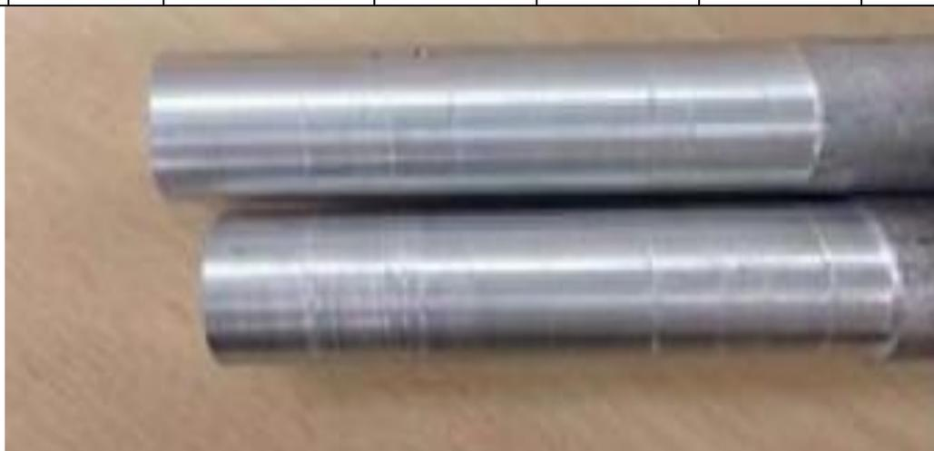
**Figure 1:** AA2219 Aluminum Alloy Matrix Composite
