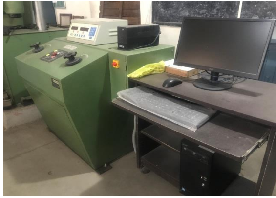
Figure 3: Universal testing machine (UTM) with PC based data acquisition system at GEC Bilaspur (India)
