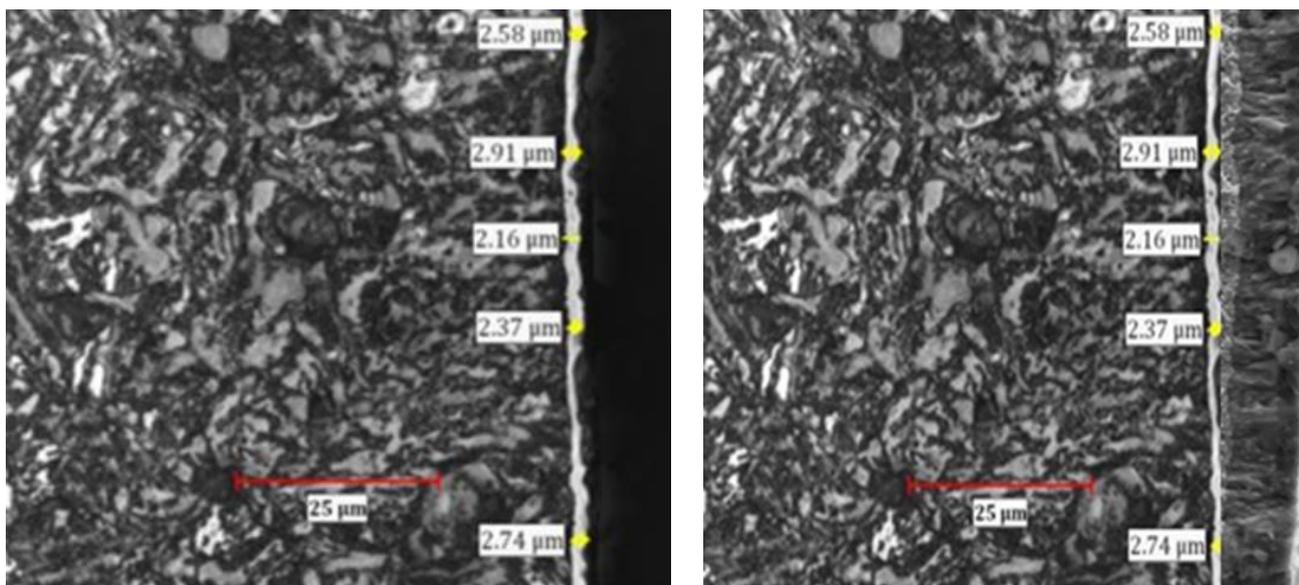
Fig. 1 Coating morphology of DLC and Ni<sub>3</sub>Al coating on ZA-27 alloy
