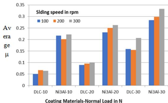
**Fig. 10** Friction coefficient of DLC and Ni<sub>3</sub>Al coating on ZA-27 alloy as function of Sliding distance and load at sliding distance of 1 km
