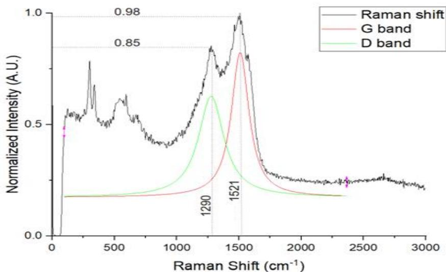
**Fig. 2 :** Raman Spectra of DLC coated on Za-27 alloy.
