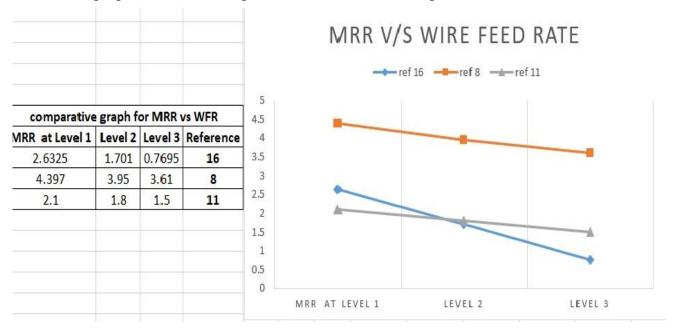
As shown in above graph we can see that as value of wire feed rate increases the material removal rate slightly decreases. it is observed that the MRR is higher both at lower and higher levels of wire feed than the canter level of wire feed. This is because increase in wire feed increases the rate of cutting speed, which in turn increases the rate of spark discharge. More amounts of material melting and erosion takes place for higher spark discharge. Hence, MRR was more at higher wire feed
