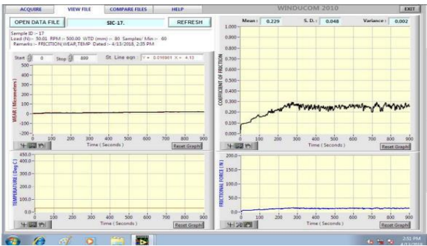
Figure 8: Result of SiC pin sample at 500 rpm and 100 N load.
