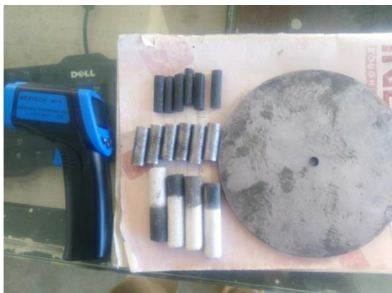
Figure 2: Silicon carbide, EN 31 Pin and disc, Infrared thermometer
