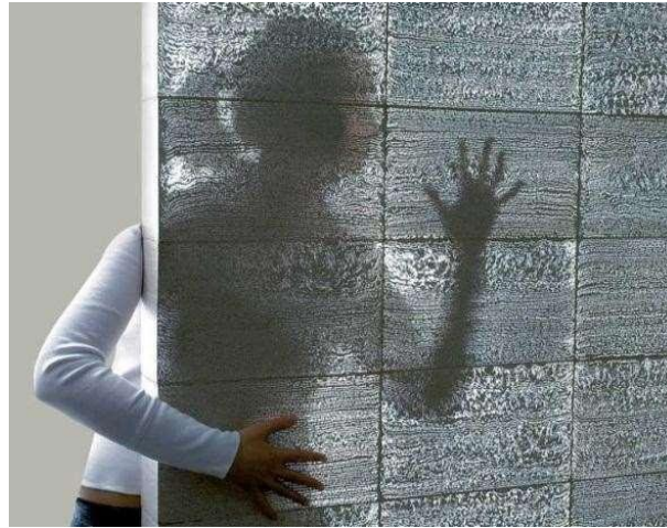
Fig 2.1 Translucent concrete wall
