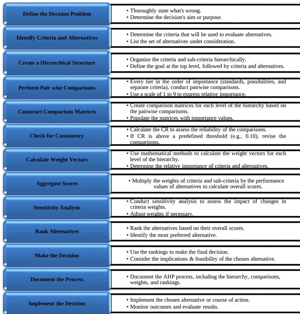
Figure 2 Flow Diagram for preparing an Analytic Hierarchy Process
