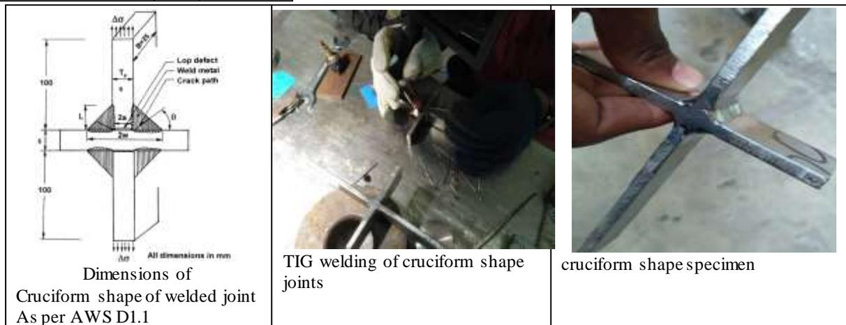
Fig 2. Fabrication of Cruciform shape weld joint
