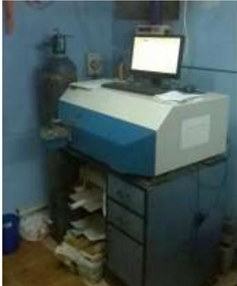
Fig.3. Optical Emission Spectroscopes
