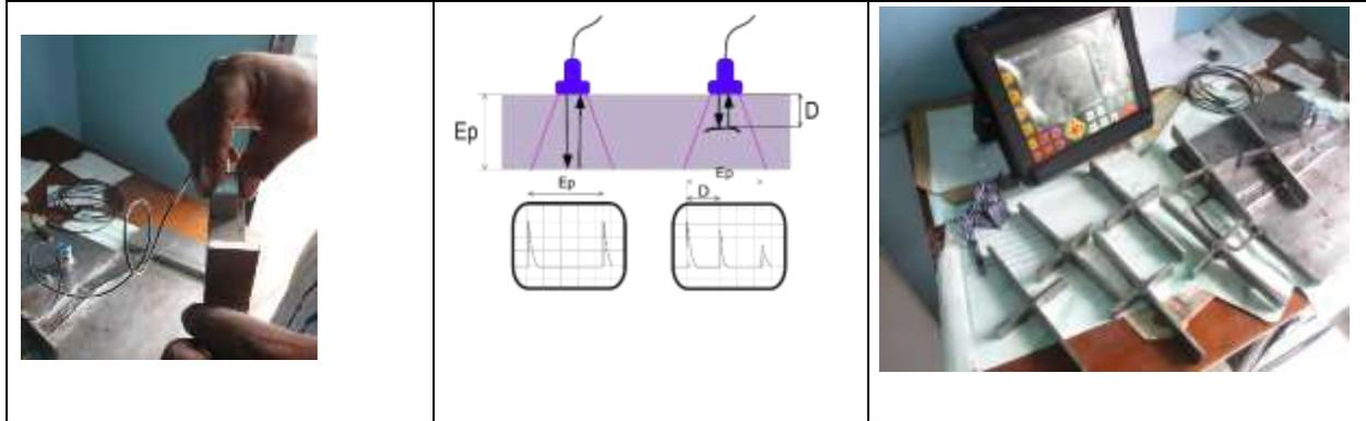
Fig 6. Ultrasonic Testing Procedure
