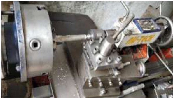
Fig.6. Machining of raw specimens
