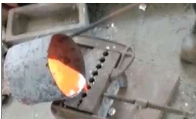
Fig.3. Pouring molten Al-TiO 2 in to the die cavity
