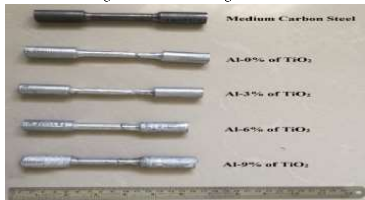
Fig.14. Tensile tested specimens after failure
