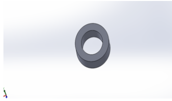
Collar part of single lap hybrid joint
