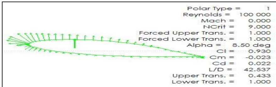
Fig 4: S822 airfoil analysis Sectionwise airfoil and its twist angle are shown in table 3.
