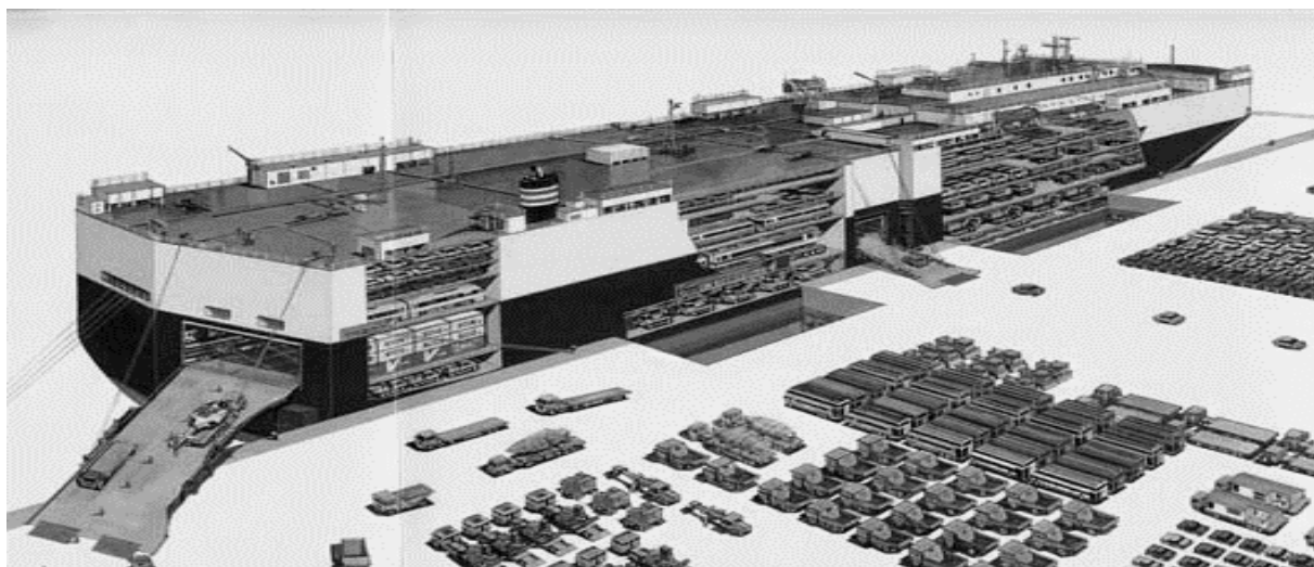
Fig 3. Ro-Ro Ship structure and cargo loading feature through the ramp
