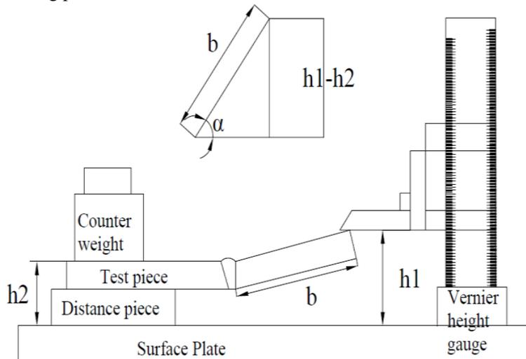
Fig. 3: Distortion was measured using a vernier height gauge.
