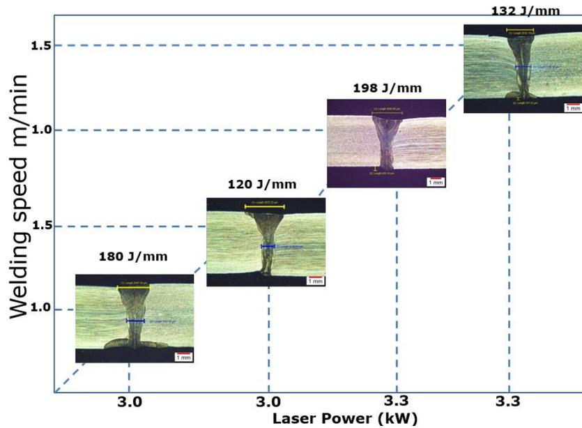
Figure 4 SS316L laser weldments macrostructure
