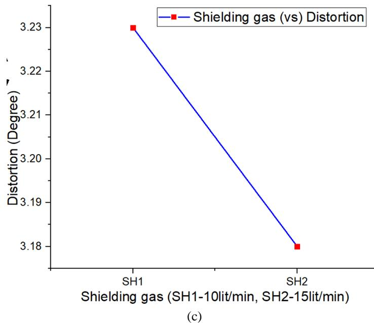
Figure 6 Effect of process parameters on distortion
