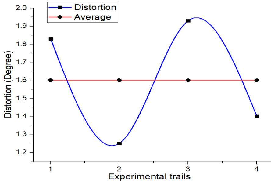
Figure:5 Distribution of distortion in the weldments
