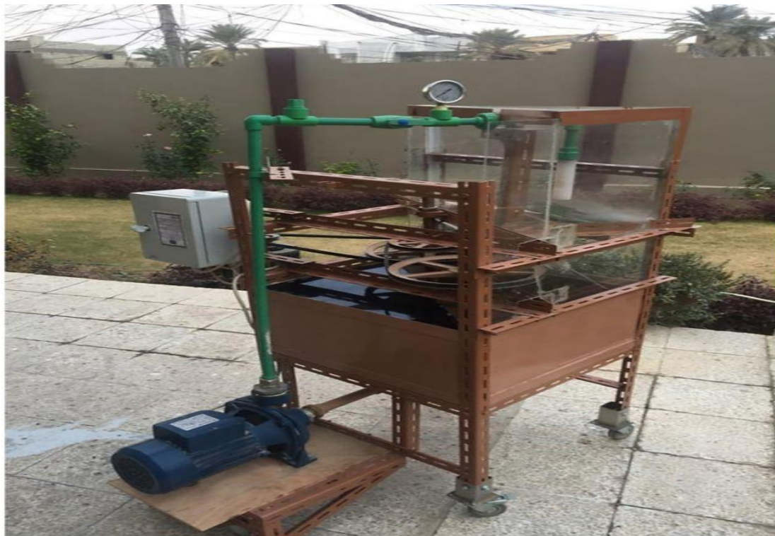
Fig. 5: erosion-Corrosion Apparatus Depend on (G73) ASTM.
