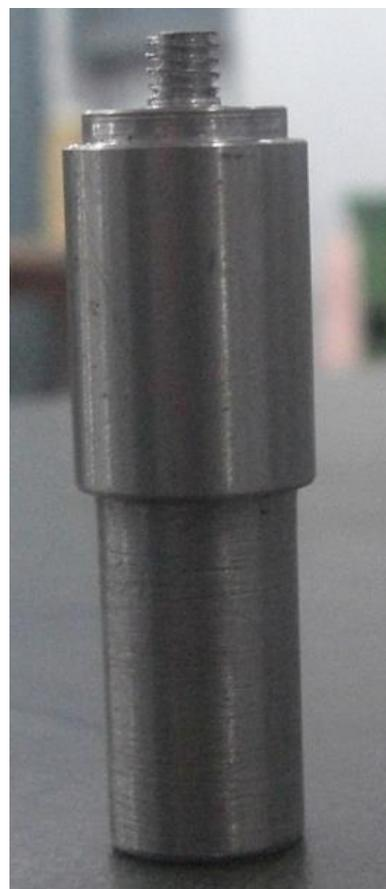
**Figure 2(b).** Cylindrical threaded pin tool
