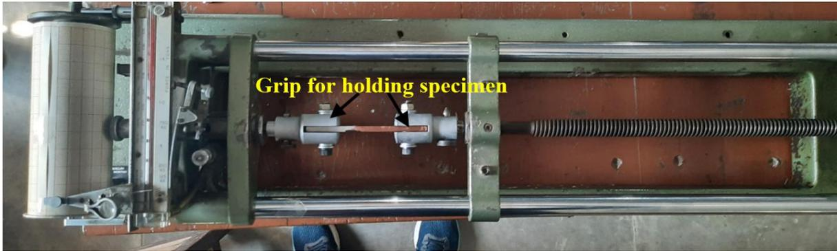
**Figure 5.** Hounsfield Tensiometer setup for performing tensile test
