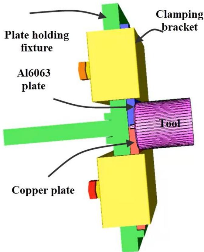
**Figure 2 (a).** Arrangement of Fixture and tool
