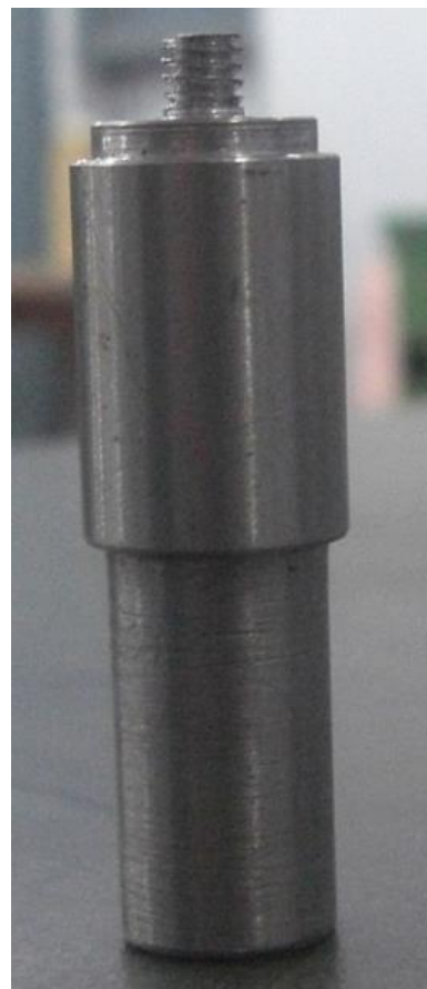
Figure 2(b). Cylindrical threaded pin tool
