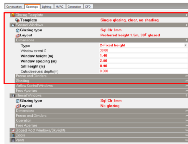
Figure 31 : The type of glass and the wall-to-glass ratio (WWR) entered to the program..
