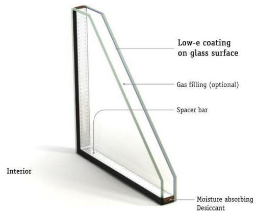
Figure 10: Layers of low-E glass.
