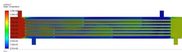
Fig. 11 longitudinal temperature contour for water with half circle baffle
