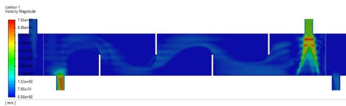
Fig. 15 longitudinal velocity contour for water with half circle baffle
