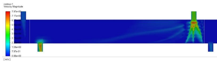
Fig. 14 longitudinal velocity contour for water without baffle
