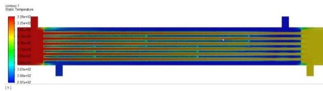
Fig. 7 longitudinal temperature contour for water with rectangle baffle
