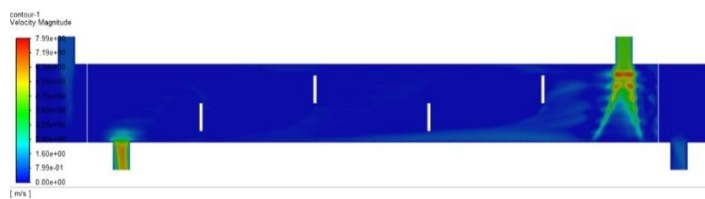
Fig. 9 longitudinal velocity contour for water with rectangle baffle
