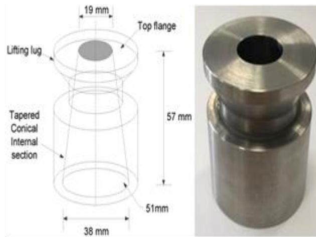
Figure 1 the mini-slump cone
