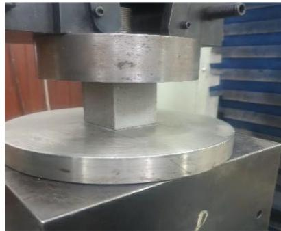
Figure 2 Compression test for test specimen using Universal Testing M/C
