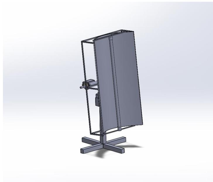
Figure (1): Solar collector with tracking system.
