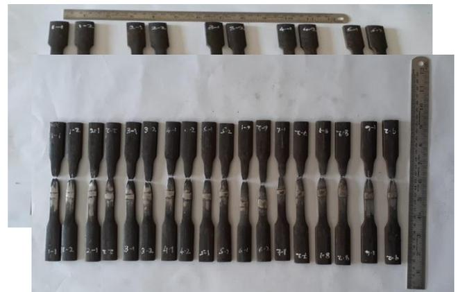
Tensile specimen samples before testing
